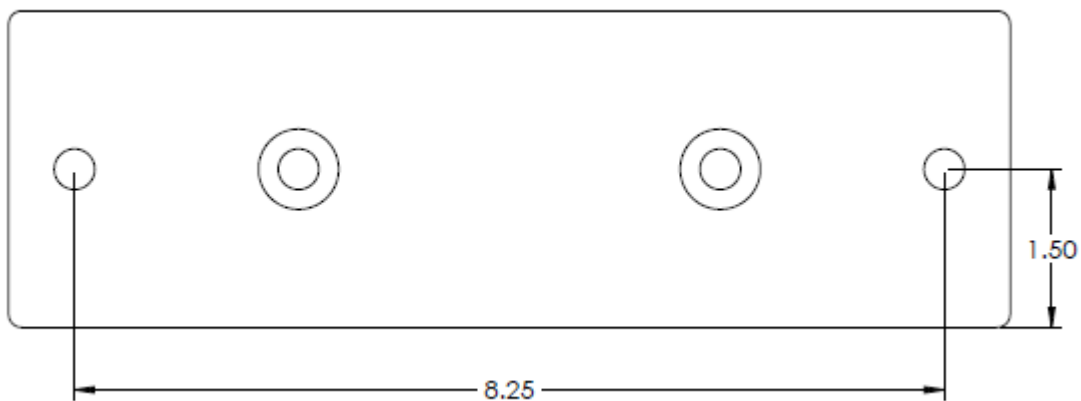
Figure 2-1 Mounting Bracket Screw Hole Locations (2)
